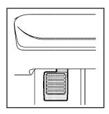
To set the parking brake, push down the parking brake pedal with your left foot. If the ignition is on, the brake system warning light will come on. See *Brake System Warning Light on page 194*.
